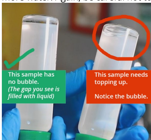
The vial on the left has no bubbles and is correct. The vial on the right has a bubble and will need to be topped up.
