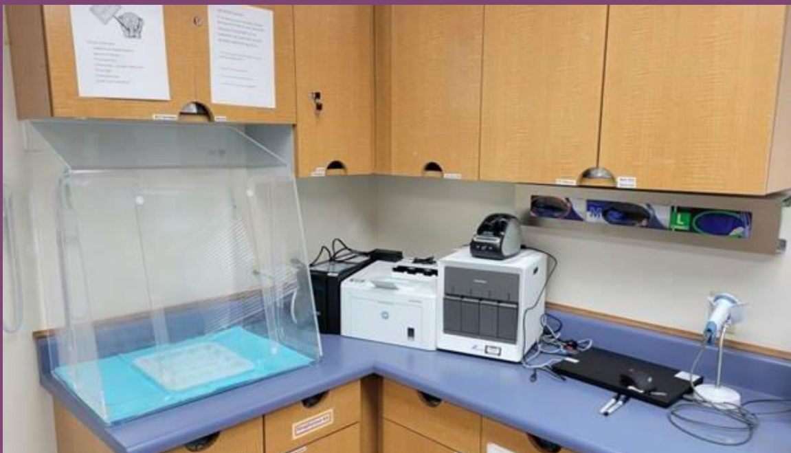
Figure 6. Sample of the Clean Spot set-up (left), later adopted for handling samples for a GeneXpert device (right of centre).
